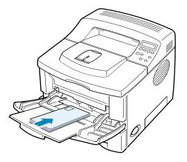
5 Adjust the guide to the edge of the envelope stack.
